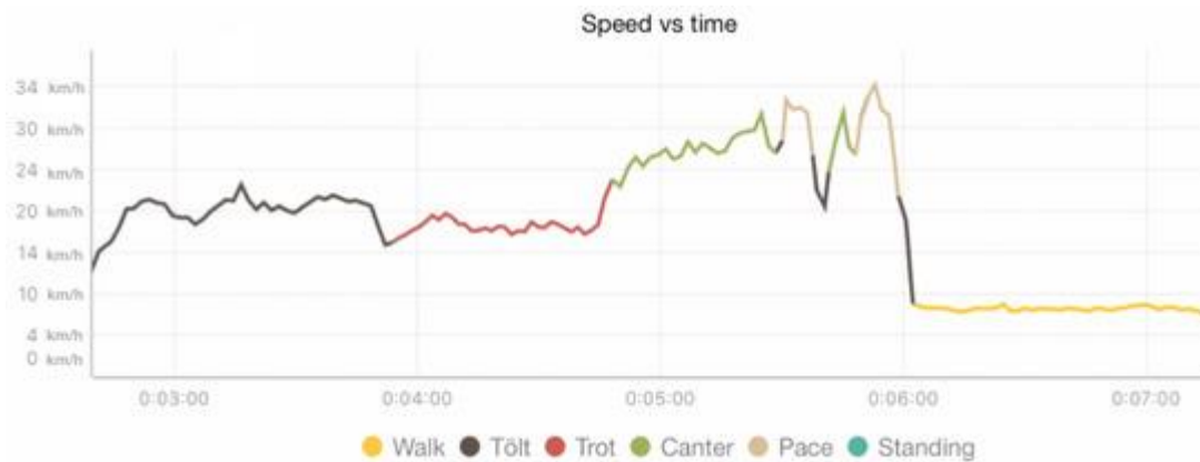
Figure 5. Plot of speed vs. time colour coded by gait from the TöltSense session overview screen
