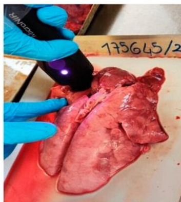
Figure 2. Recording of NIR spectra from porcine lung tissue using a portable handheld spectrometer.
